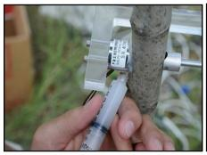
5. Apply silicone grease for a gastight seal around instrument.
