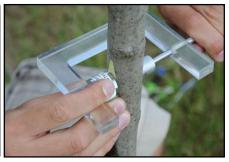
4. Secure sensor flush against plant using clamp.
