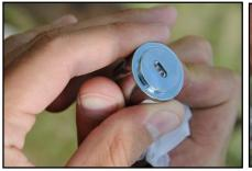
1. Make sure sensor is clean & thermocouples are intact.
