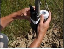
6. Attach automated PSY data logger to plant.
